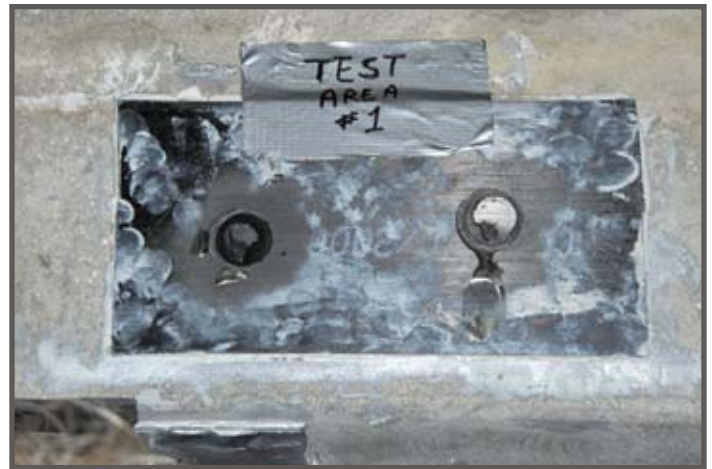
Performing pull tests by a certified testing agency are essential in ensuring the desired bond line adhesion which is critical for the intended application’s performance.
